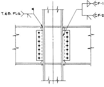
WEB BOLTED - FLANGE BUTT WELDED
