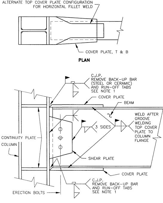
NOTE 1. GRIND SMOOTH TO REMOVE STRESS RISERS AND LAYER OF MARTENSITE FROM BURNING OPERATION
